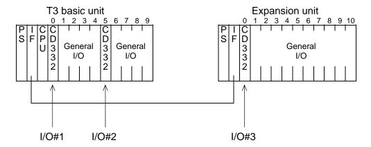
As for the interrupt priority, the interrupt generation module which is allocated closest to the T3 CPU has highest priority and followed by this order.
